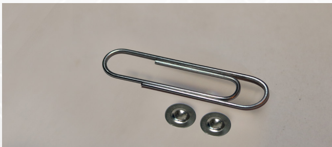
1/8 in (3mm) nominal size FRB disk adjacent to a standard sized paper clip.
